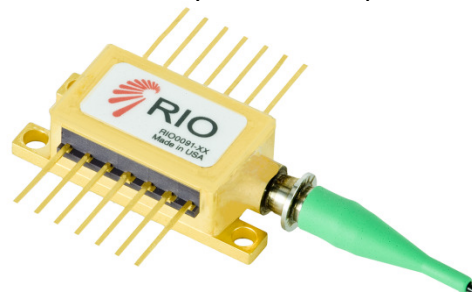
Figure 2. RIO ECL 009x laser in 14-pin Butterfly package
